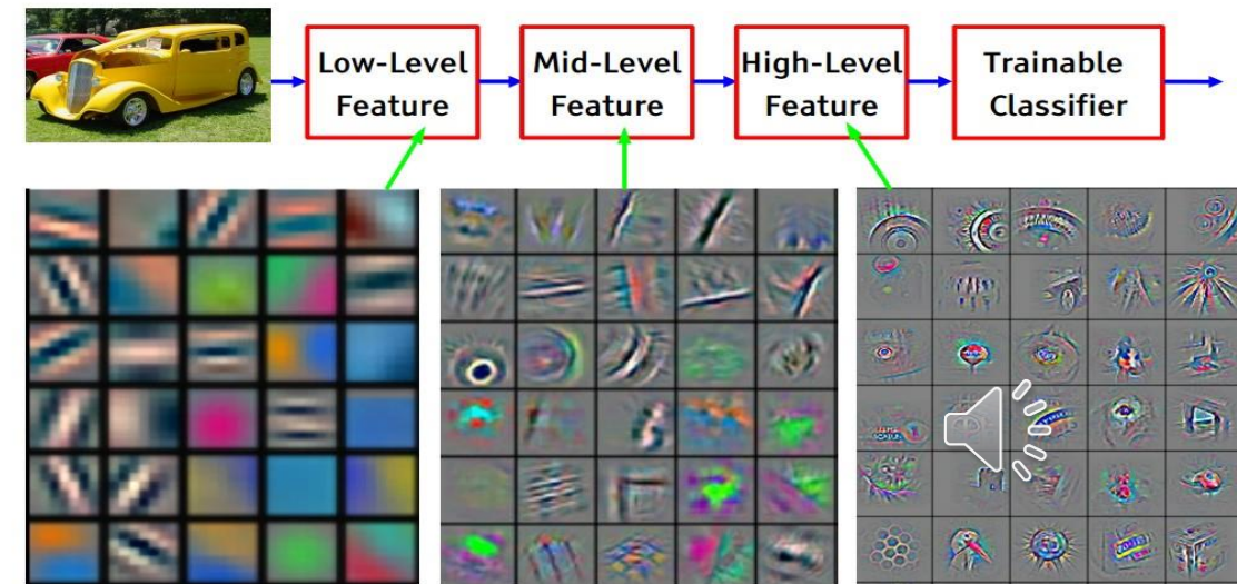
Feature visualization of convolutional net trained on ImageNet from [Zeiler & Fergus 2013]
