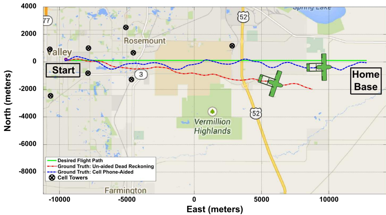
Figure 25: Extended HIL Simulation: Comparison of North and East Estimated Positions
