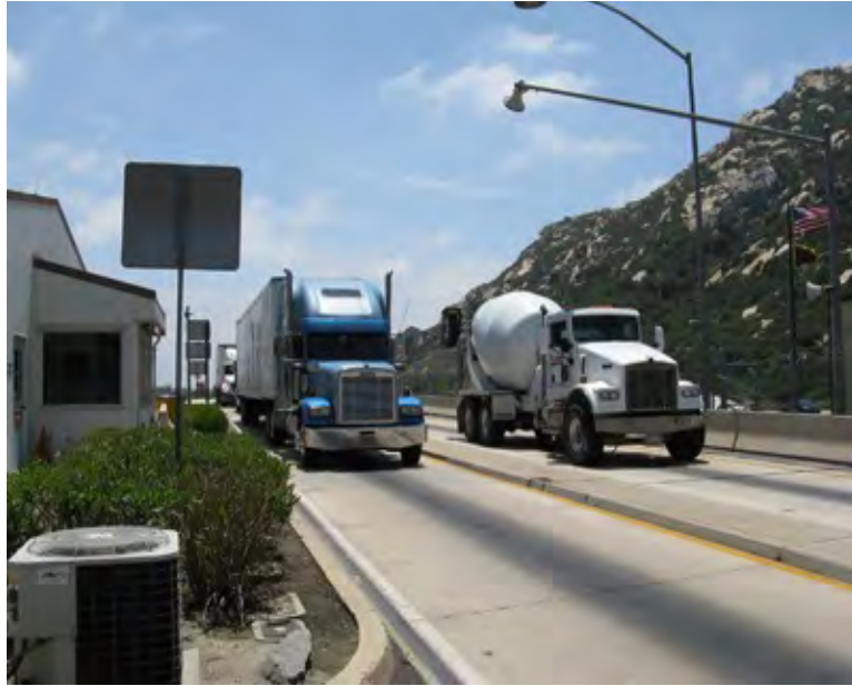
Figure A.27. I-8 checkpoint screening operations of commercial vehicles at the adjacent CA weigh station. Continuous commercial vehicle screening is possible even when the general public lanes must be flushed. (Source: UA)
