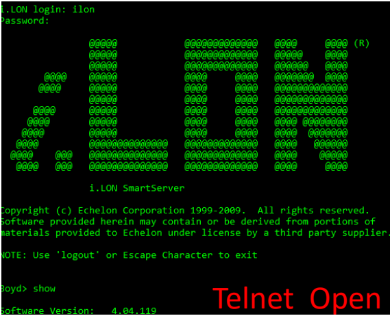
Figure 8: Example of vulnerable SCADA device on Telnet
